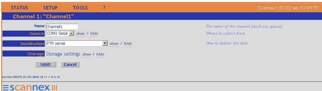
The screenshot shows the 'Channel 1: "Channel1"' configuration page. The 'Name' is 'Channel1'. The 'Source' is set to 'COM1 Serial'. The 'Destination' is set to 'FTP server'. There are 'Storage settings' and 'SAVE' and 'Cancel' buttons at the bottom. A footer note says 'Version IPBCF2.30.105 2008-12-11 / 15.0.10' and the Scannex logo is at the bottom.
